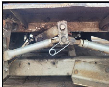
"Improper Toggle Arm Hardware/ Loose Adjusting Nut"
