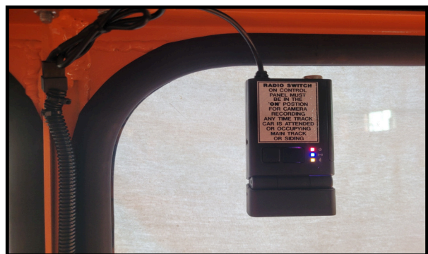
Outward Facing Camera Installed
