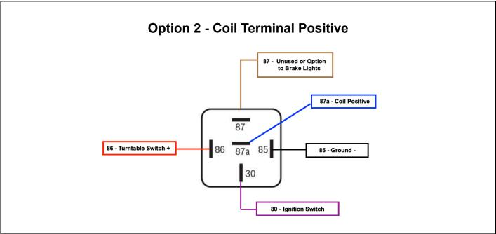
NOTE: Make sure to use a 5 Pin Relay with separate 87 & 87a pins.
