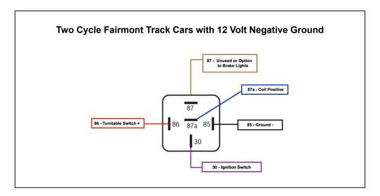
NOTE: Make sure to use a 5 Pin Relay with separate 87 & 87a pins.
