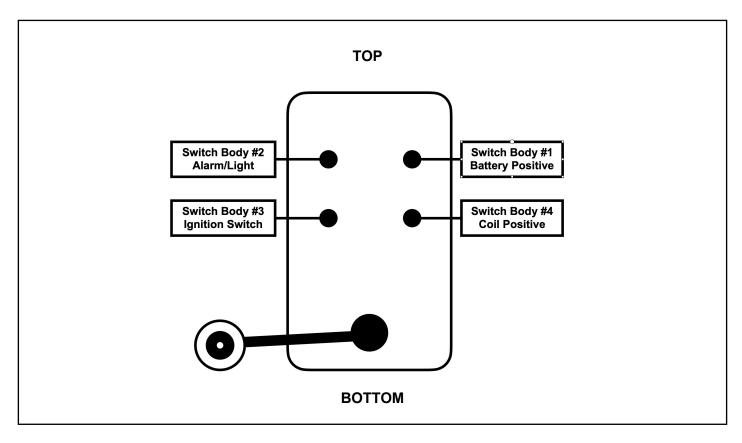
Note: #1 and #2 - Normally OPEN when turntable is fully retracted. #3 and #4 - Normally CLOSED when turntable is fully retracted.
